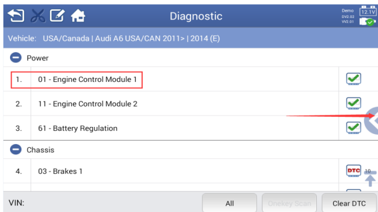
Figure 4-11-1 Electronic Control System Menu.
