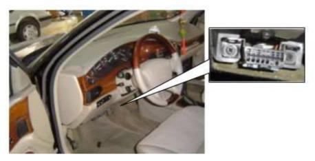
\*GM Buick: the OBD plug is below the dashboard, use SMART OBDII-16 connector.
